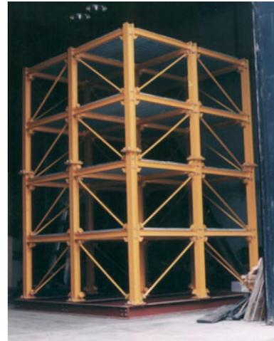
**Fig. 4.** Benchmark test structure (Structural Health Monitoring Benchmark Problem).
