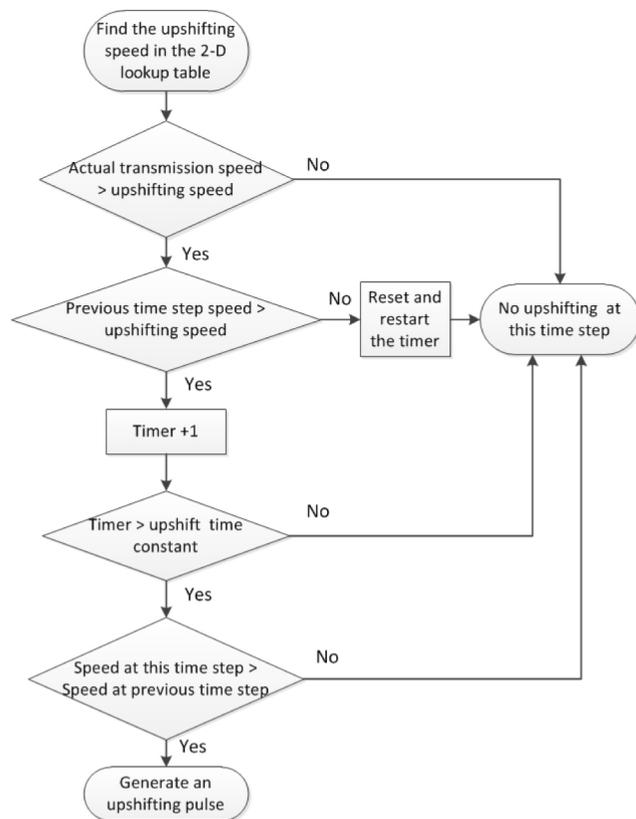
Figure 7. The flowchart of upshifting control.
