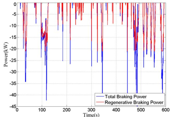
Figure 14. Braking power in US06 drive cycle.
