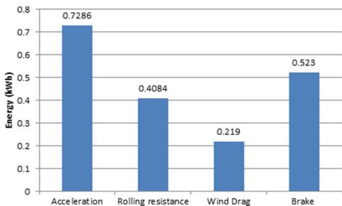
Figure 13. The breakdown of traction energy over a UDDS drive cycle.
