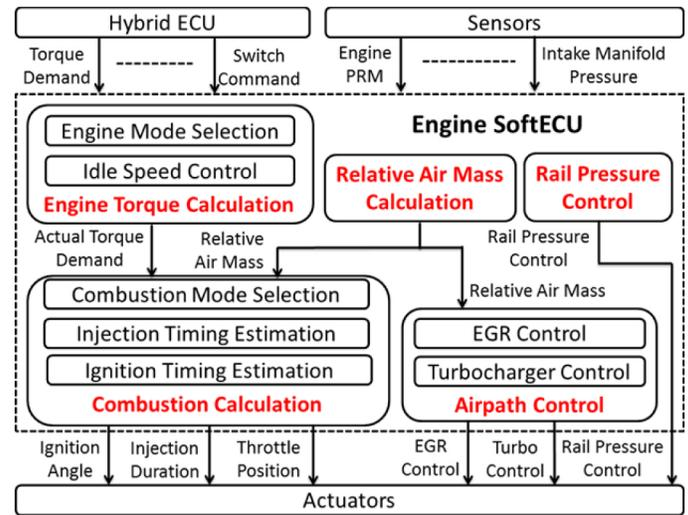
Figure 5. The block diagram of engine ECU.
