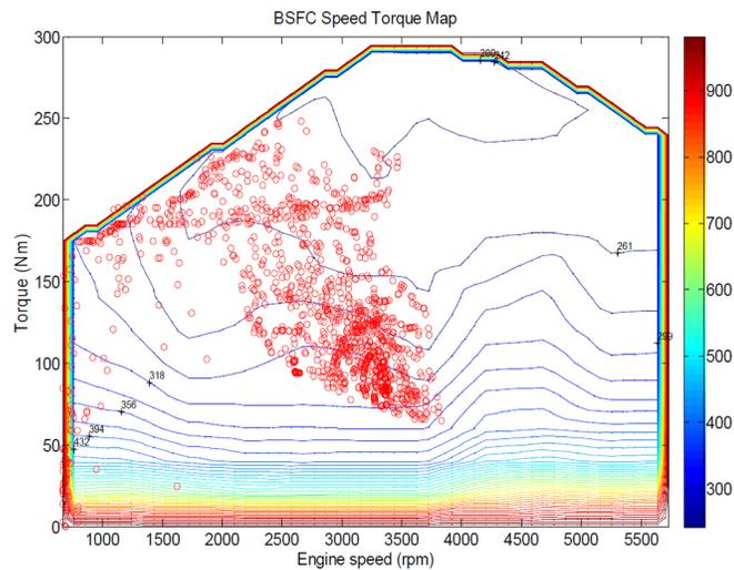
Figure 16. BSFC speed torque map for engine in HEV running on UDDS.
