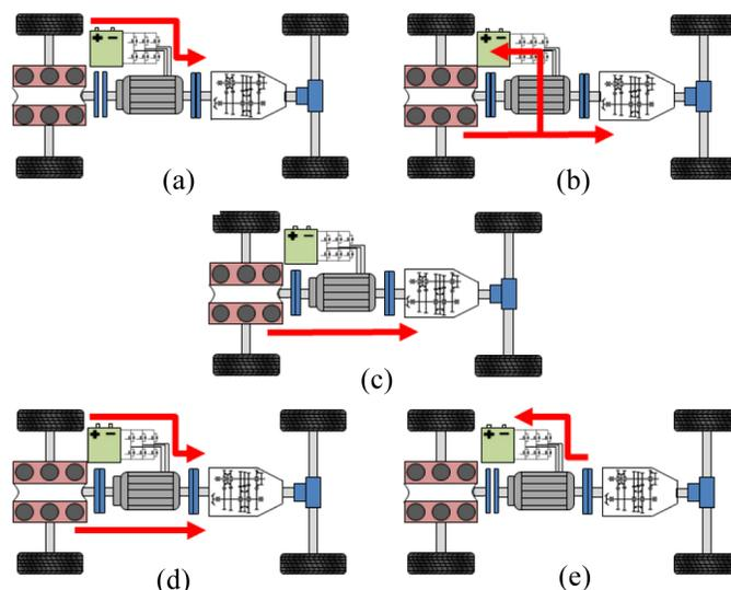
**Figure 3. Vehicle operation modes and powertrain energy flow. (a) Electric only mode. (b) Battery charging mode. (c) Engine only model. (d) Hybrid mode. (e) Regenerative braking mode.**
