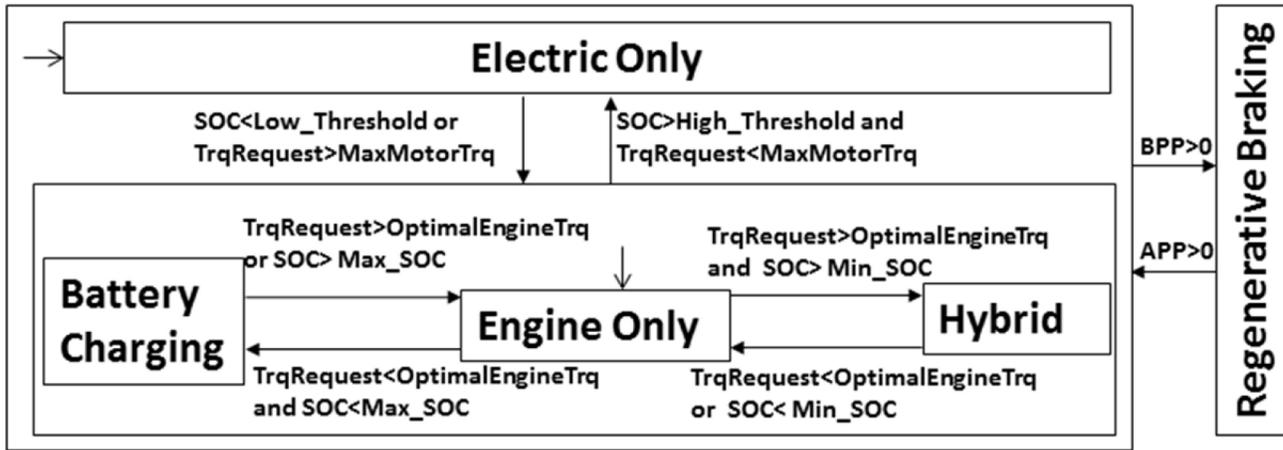
Figure 4. Vehicle operation mode control and transition conditions.
