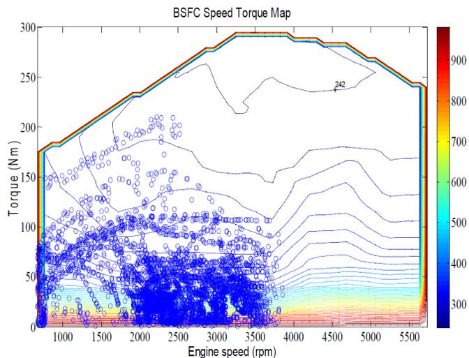
Figure 17. BSFC speed torque map for engine in conventional vehicle running on UDDS.
