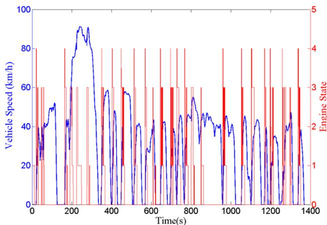
Figure 15. Engine states in UDDS drive cycle.
