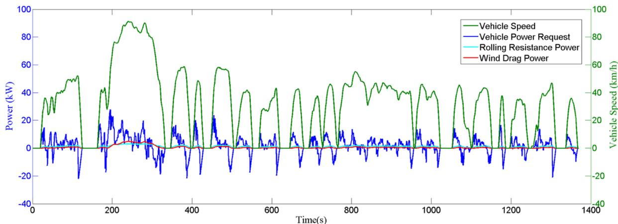
Figure 12. Vehicle power request, rolling resistance power, and wind drag power over a UDDS drive cycle.
