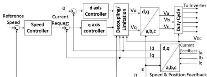
Figure 6. The block diagram of motor ECU.
